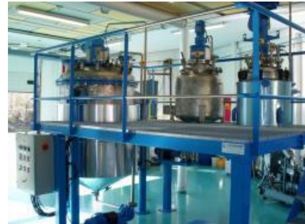
Figure 1 Autoclave reactors used for the production of the sorbent and catalyst support powders
