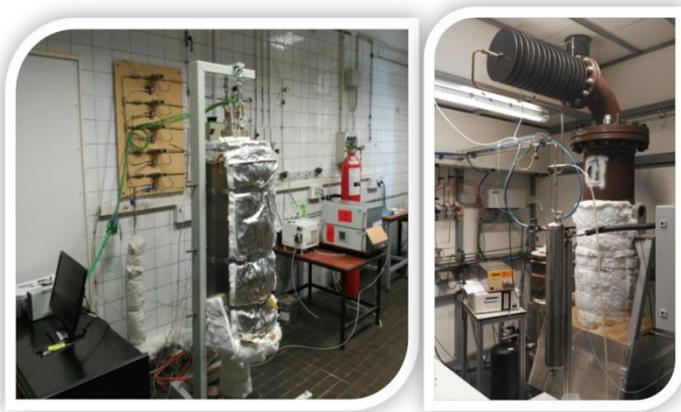
Two experimental test rigs for the investigation of the CaCu cycle
